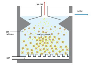
Figure 27. Diagram of a UASB Reactor
