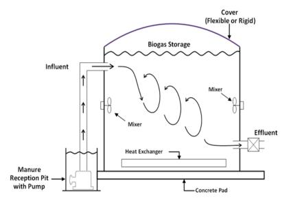
Figure 23. Diagram of Completely Mixed Digester
